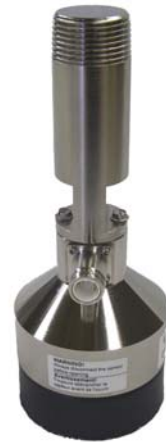
Fig. 2 This shows the SR50A/AT Mounting Stem attachment (008164) fitted to the SR50A/AT sensor body
