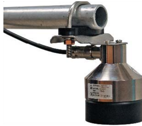
Fig. 1 The 19517's bracket mounts directly to a crossarm. Two screws are used to attach the SR50A/AT to the 19517 bracket.
